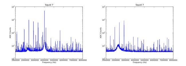
In the left plot the squid had been tuned in the regular fashion with 10K feedback. In the right plot the squid has been set to openloop. Opening the loop doesn't seem to have much effect on the forest, however it does have a detrimental effect on the peak at  $\sim 2.3$  M Hz.
